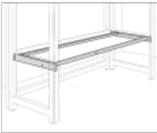
Stretcher & Reinforcement Bars
